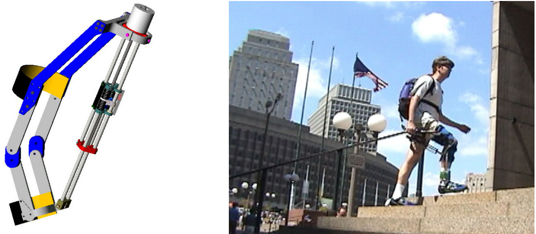
Figure 7: The RoboKnee, an exoskeleton for enhancing human strength and endurance. CAD rendering (left) shows the knee brace and electric Series Elastic Actuator. A single RoboKnee (right) assisting the author in climbing steps.
